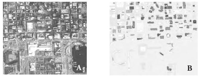
Figure 1. Test data for downtown Baltimore. A: Orthoimage. B: Color-coded lidar grid. (light: low elevation; dark: high elevation).
